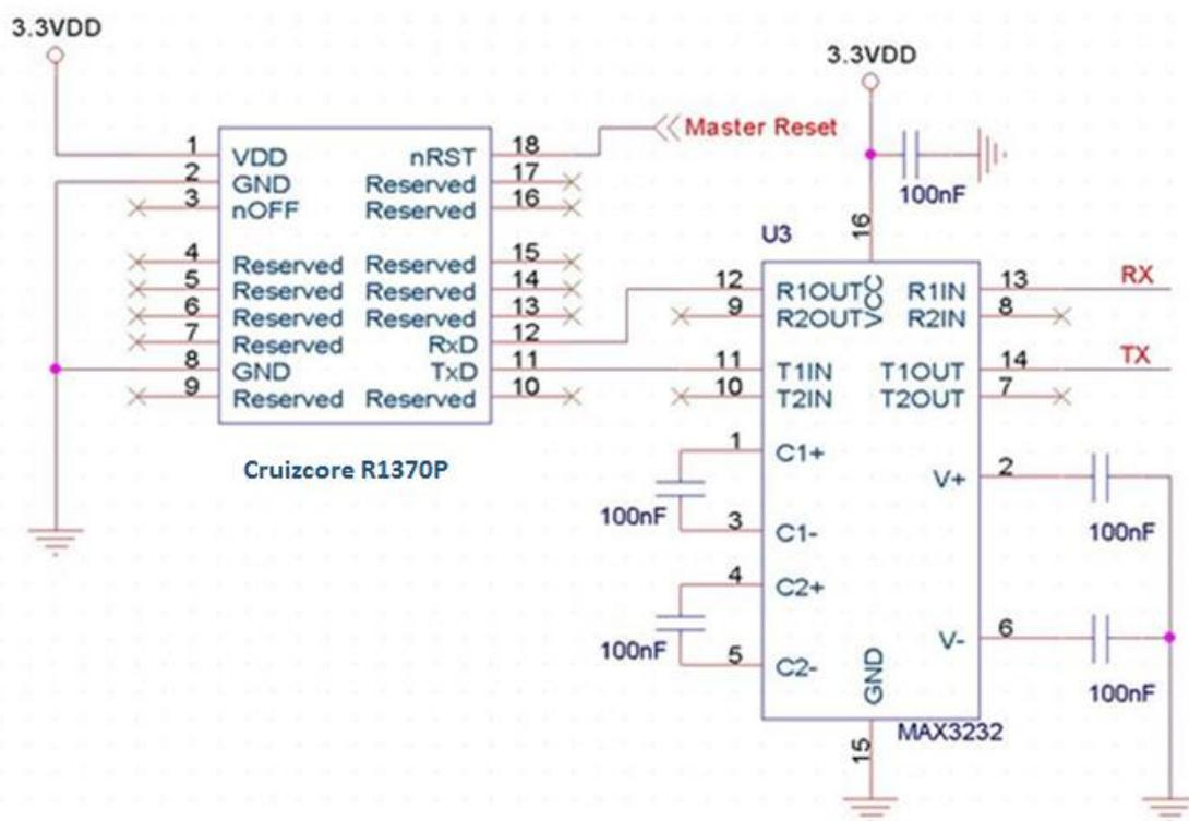
Figure 9: CruizCore® R1370P with RS232 level converter
