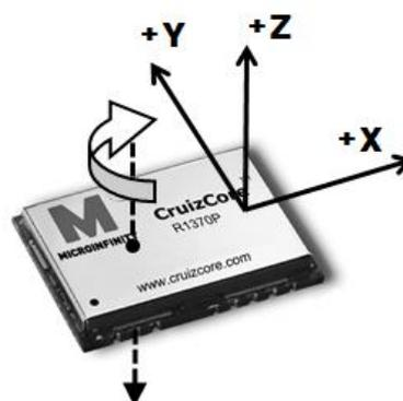
Figure 4: CruizCore® R1370P coordinates system
