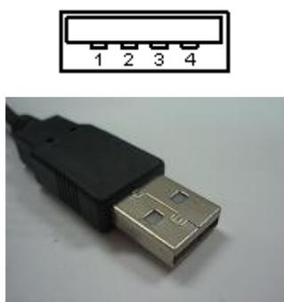
Figure 3: Type A USB connector.
